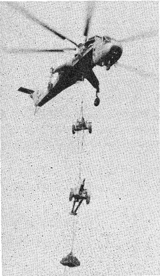
You call, we haul! A CH54 of the 478th Avn Co, 34th Med Bn lifts two 105mm howitzers and an ammunition bag for the 2/10th FA during the FTX, Operation Indian Village I.
